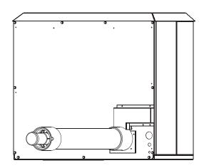
Step 6. Direct vent co-axial venting is completed.
